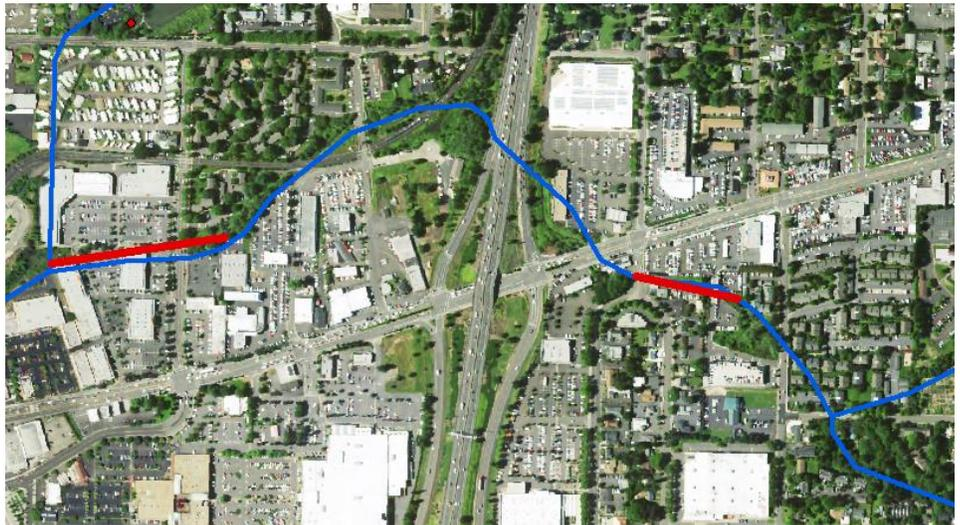
Figure 3. The river segment shown in blue was culverted. Red lines overlay sections of the river under parking lots or commercial infrastructure.
